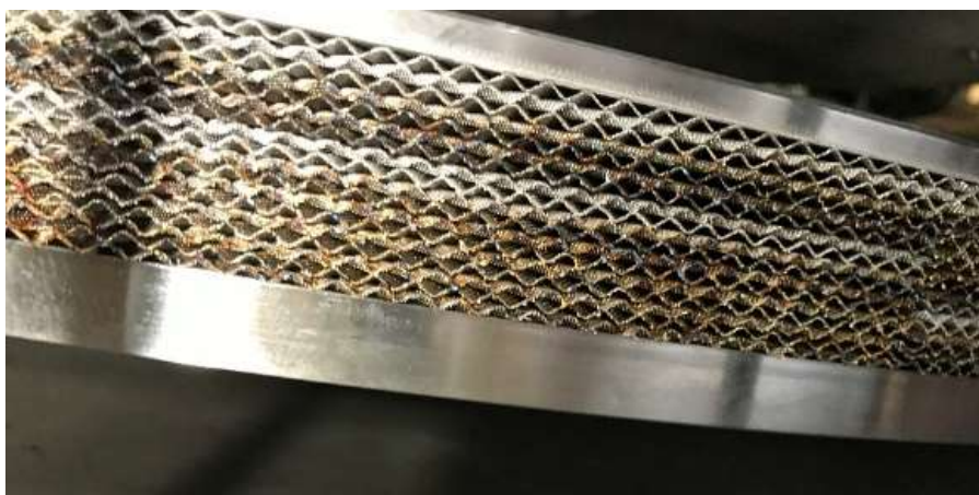
Figure 13. Closeup of Absorber Rotor with Packing.
