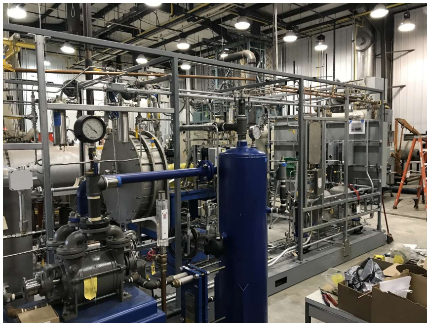
Figure 19. ROTA-CAP Test Skid and Blower Skid.
