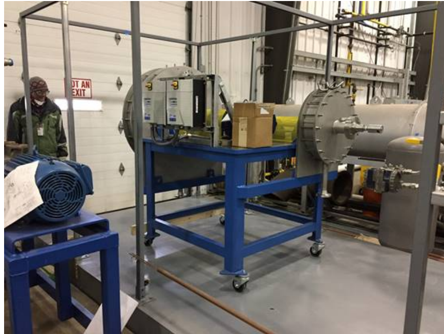
Figure 17. RPB Assembly Located on the Skid.
