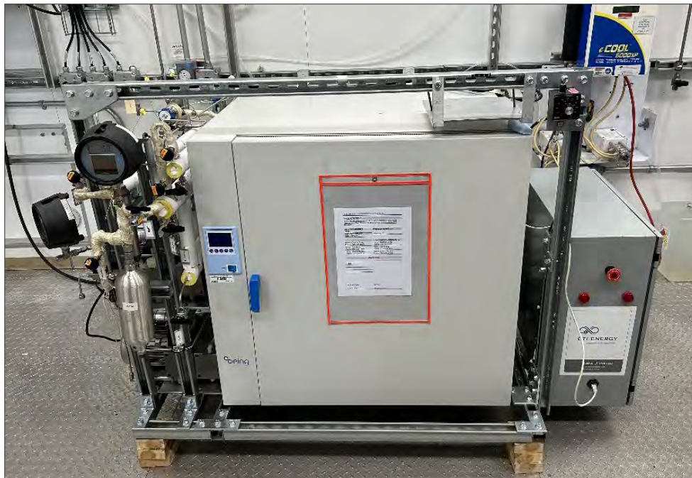
Figure 17. GTI Energy Graphene Oxide-Based Membrane Test Skid Installed in LSTU
